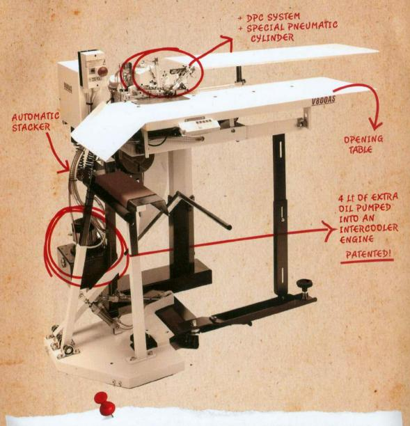
Equipped with a super fast Yamato sewing head fully made in Japan, the V800AS is a 2 needle, 4 thread overlock unit that runs at 6300 rpm (maximum speed 7000 rpm).
