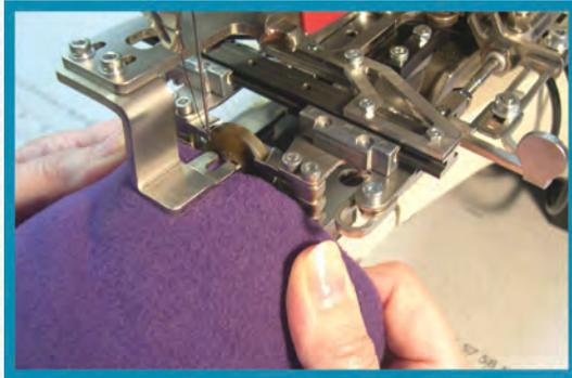
precisely adjustable back stop and simple garment loading
