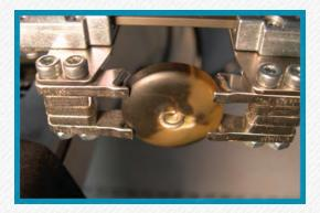
Unique linear clamping button holder means holding large or small buttons can be achieved with no adjustment
